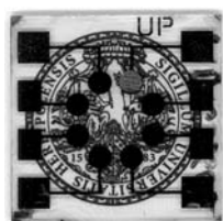
Figure 3. Picture of a transparent device containing a blend of 10c :PC 61 BM (25/75 wt %) lying on the seal of the Universität Würzburg.
